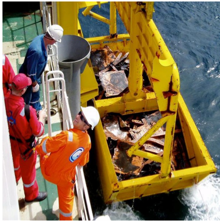
A 100 ton skip is being raised on board Ship containing many tons of copper ingots.
